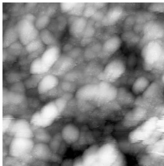
Fig. 5 STM image of one electrode of a membrane electrode (MEA) with carbon supported Pt 1 \text{ mg cm}^{-2} catalyst in 0.1 \text{ mol L}^{-1} \text{ H}_2\text{SO}_4 , U = -0.1 \text{ V} , I_{(\text{tip})} = 1 \text{ nA} , image size 100 \text{ nm} \times 100 \text{ nm}
